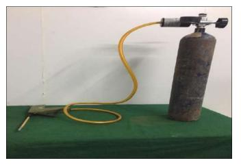
Fig 3: Liquid nitrogene oxide cylinder with cryo probe.
